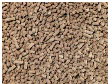
Figure 9 - Fertilizer produced from sewage sludge ash treated by the ASH-DEC process (Adam 2008)
